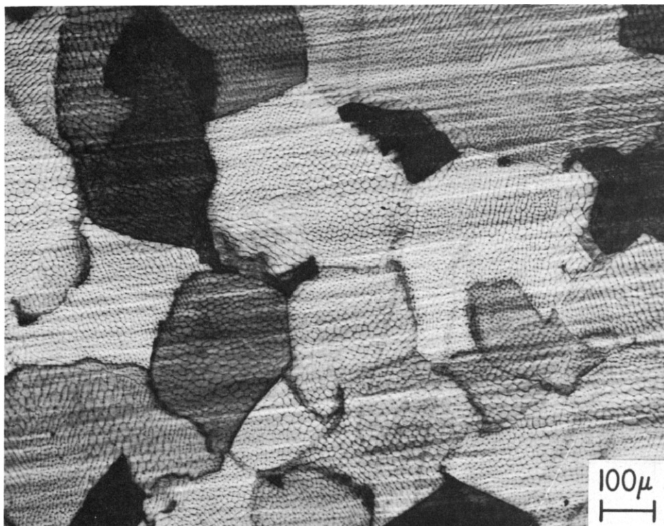
Fig. 4. Chill-cast ternary alloy Pb-0.053 Ca-0.70 Sn; 100X. Regular hexagonal subgrains viewed in direction of solidification.
