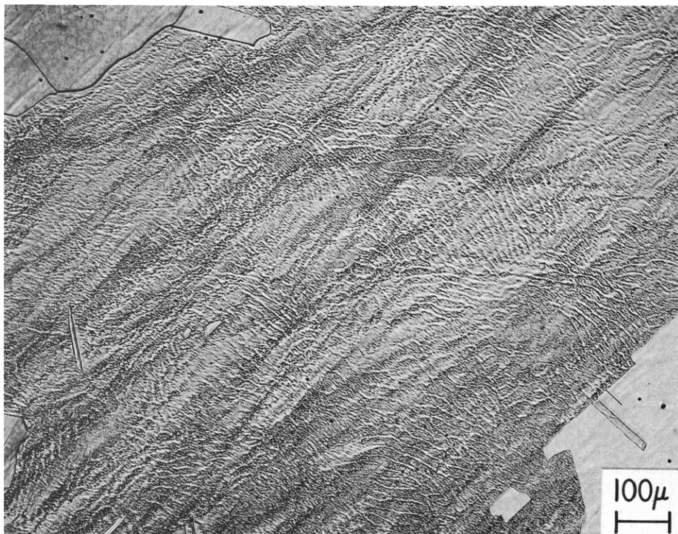
Fig. 3. Chill-cast pure Pb; 100X. Note irregular subgrains consisting of convection cells.
